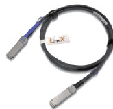
Direct Attach Cables (DACs) • 400Gb/s, NDR(400G) • 200Gb/s, HDR(200G)
